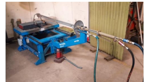
Oxyfuel prototype to evaluate the use of H 2 in metallurgical cutting.
