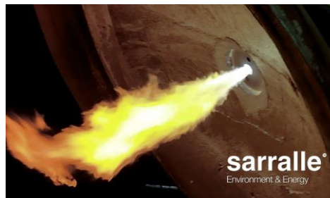
First spoon heater capable of running entirely on green H 2 .
