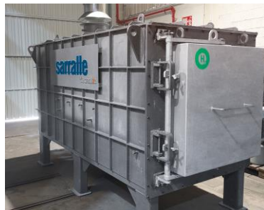
Reheating furnace prototype for the evaluation of hydrogen combustion technologies.
