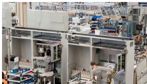
Manufacturing of a new rectifier solution for powering electrolyzers based on IGBT technology.
