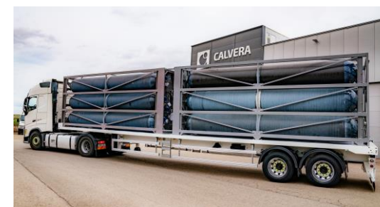
The world's largest tube trailer in terms of pressure (517 bar) and capacity (1.3 ton) for hydrogen transport.
